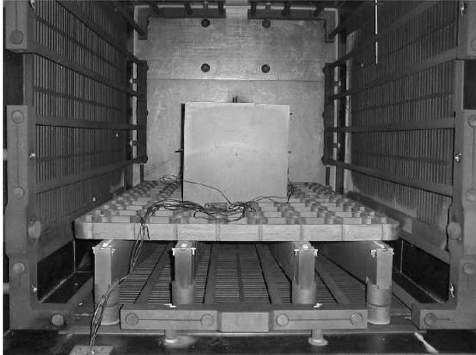
Figure 4. FORD / GMPD Specimen  $400 \times 400 \times 400$  mm in furnace.
