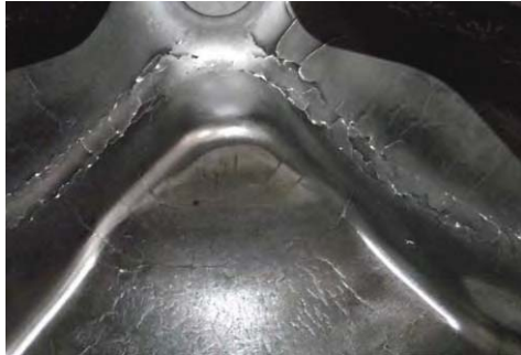
Figure 2. Surface of an aluminum part which was cast in a die having cracks in the mold. Source: Price [34].
